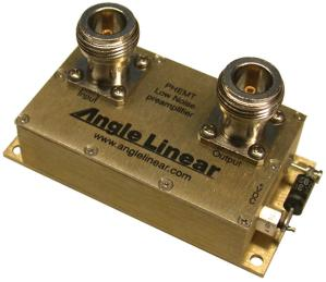
Every preamplifier has over and reverse voltage protection. External and internal high voltage transient suppressors provides 40kV, 1 micro sec. pulse protection. Internal voltage regulation permits operation from +11 to +28 VDC. For voltages greater than +18 VDC an external dropping resistor should be employed. Filtering on the DC terminal provides >70 dB attenuation from 20 MHz to several GigaHertz. DC current requirement is typically 100 mA.
