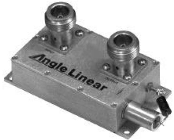
Every preamplifier has over and reverse voltage protection. External and internal high voltage transient suppressors provides 40kV, 1 micro sec. pulse protection. Internal voltage regulation permits operation from +9 to +18 VDC with higher voltage options available. Filtering on the DC terminal provides >80 dB attenuation from .5 MHz to several GigaHertz. DC current requirement is typically 30 mA per amplifier stage.
